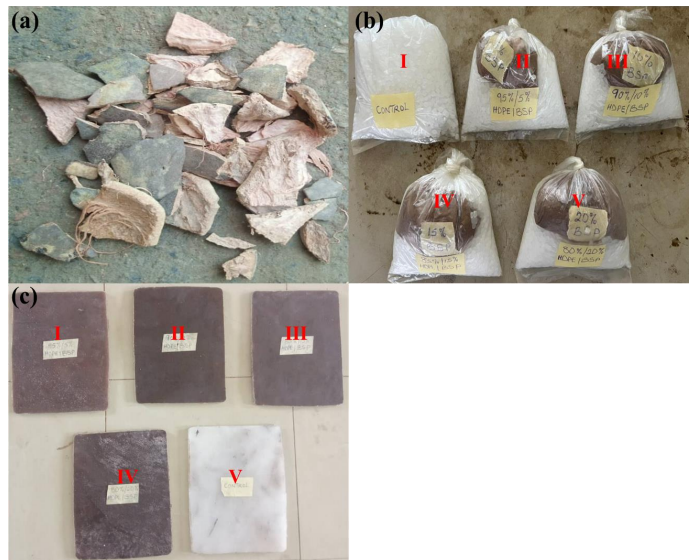
Figure 3. (a) Reduced size baobab shells; (b) Prepared composition of BSP/HDPE for (i) 0:100wt%, (ii) 5:95wt%, (iii) 10:90wt%, (iv) 15:85wt%, and (v) 20:80wt%; (c) Produced rectangular composite sheet of BSP/HDPE matrices for (i) 5:95wt%, (ii) 10:90wt%, (iii) 15:85wt%, (iv) 20:80wt% and (v) 0:100wt%.
