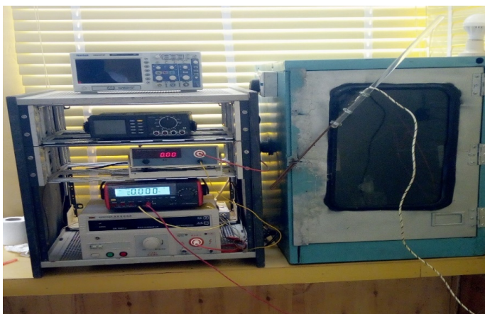
Figure 5. Dielectric-breakdown measurement setup.
