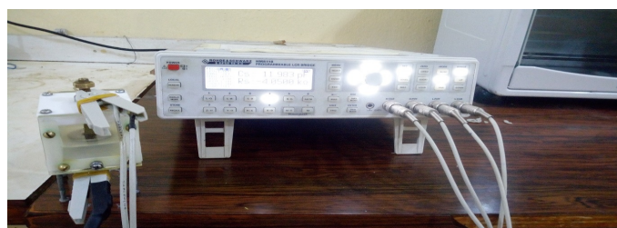
Figure 4. Rohde & Schwarz HM8118 programmable LCR bridge.
