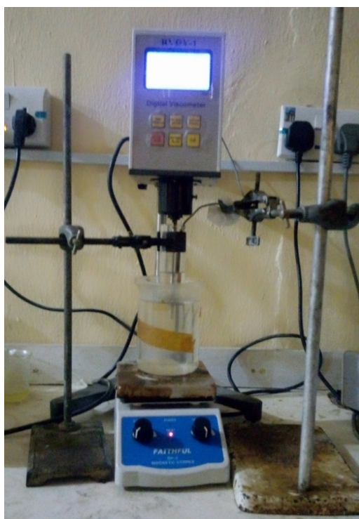
Figure 3. Viscosity measurement setup.
