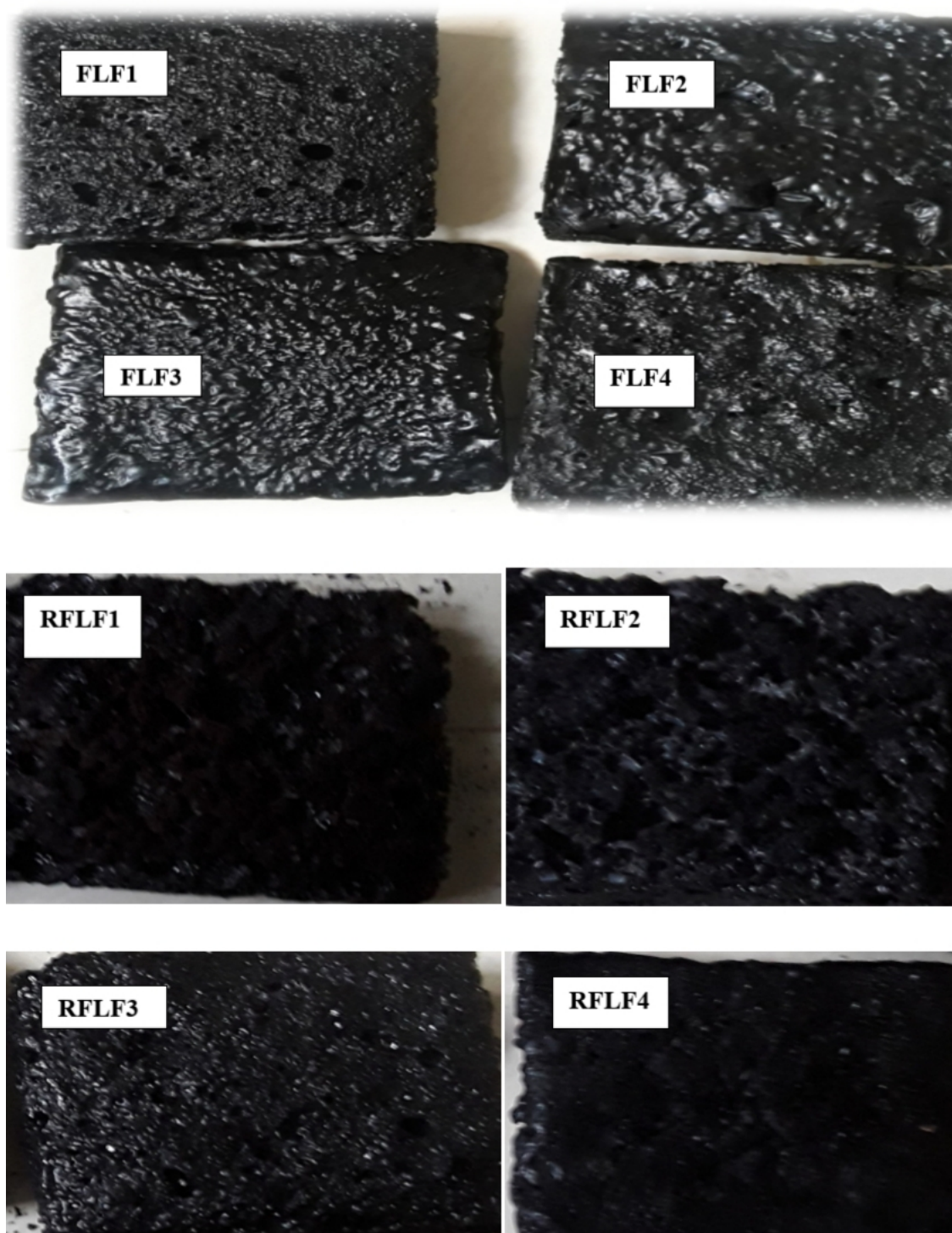
Figure 2. Image-based assessment of recycled furan–lignin foams and virgin foams prepared using the formulations in Table 1.
